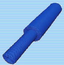
Model of Multi-Wall CNT
