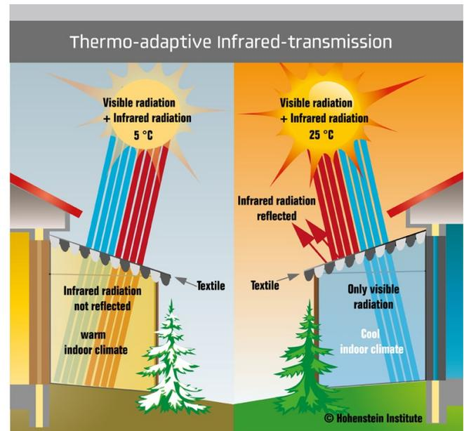
Figure 1: Intelligent textiles which are not only translucent but also able to adapt their thermal permeability to suit the ambient temperature, have the potential of significantly cutting the cost of heating and/or air conditioning. – Source : Hohenstein Institute
